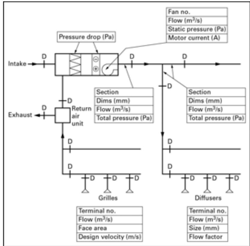
**Figure 1:** Basic schematics for system regulation showing damper positions.
