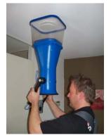
The **AT-242** is required for measuring supply vents in the housing industry.
