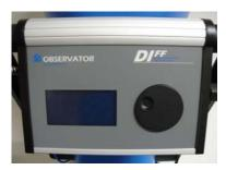
The DIFF can be switched on by pushing in the <u>middle</u> of the scroll button. The recess in the scroll button is intended for scrolling.
