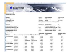
The header of the report can be customized to the style of the company. To change the header you should place a picture called diffheader.jpg in the DIFFiner folder. The header will now change into the picture called diffheader.jpg. The folder DIFFiner can normally been found in C:\Program Files\Observator\DIFFiner or on the SD-card. It is recommended to keep the same resolution as the default header (800 x 120) to avoid lay-out changes.
